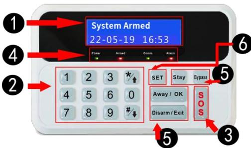
A Schematic diagram of LCD control keyboard
